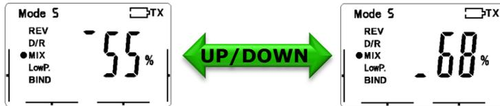
*i* Ailerons move in the same direction (Flaps) when the CH6 switch is activated (set up)
