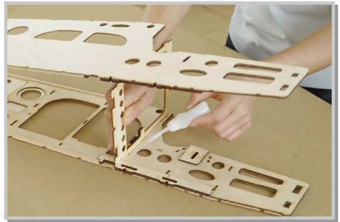
1.12 Take F5 and latch between the panels. Make sure the side with glued plywood block is facing the rear. Apply a few drop of CA to temporary fix its position perpendicular to the left side panel.
