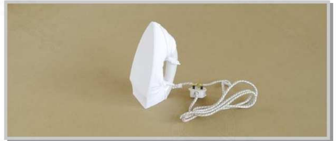
11.1 Cover iron with cotton cloth to eliminate scratch and better temperature distribution. A hobby grade sealing iron with cover sock is recommended for better handling.
