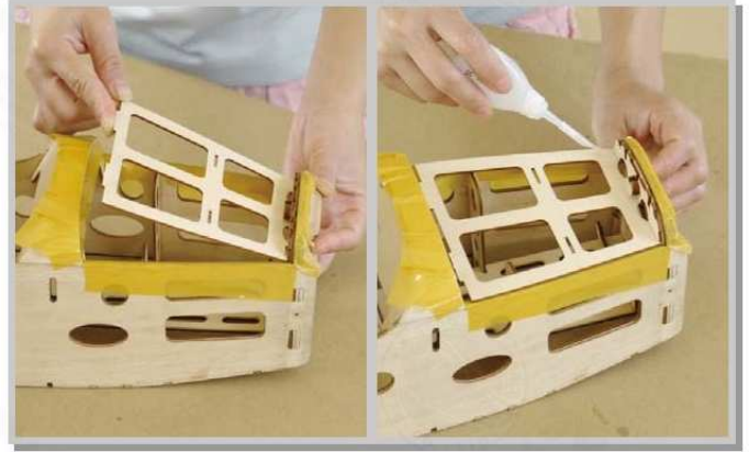
5.3 Latch in F35, apply CA to glue it in place.
