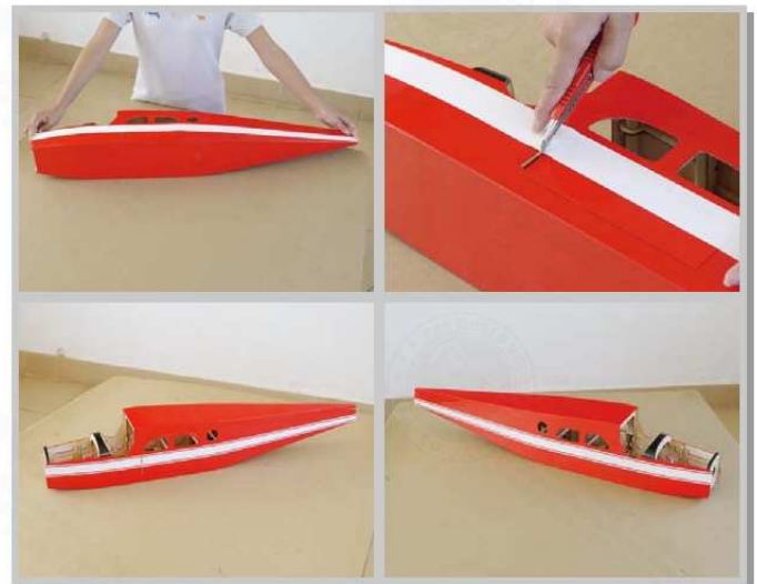
11.11 Iron on the side color trimming. Tack both ends of the trimming stripe to fix the position before ironing.
