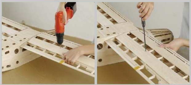
10.4 Use the pre-drill hole at W4R as guide, drill 3/32 in. hole through wing tube. Use PA3x20mm screw and washer to fasten the wings.
