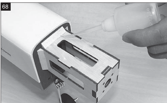
68 Glue the three hard wood by epoxy glue.
