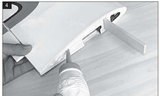
Apply the epoxy into the wing section.
