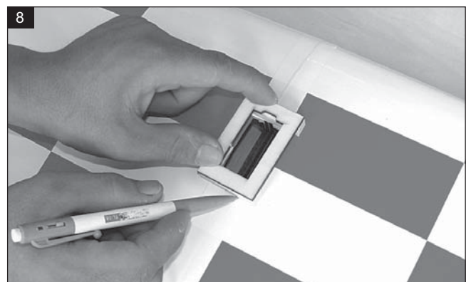
Mark the shape of the servo box to the wing.
