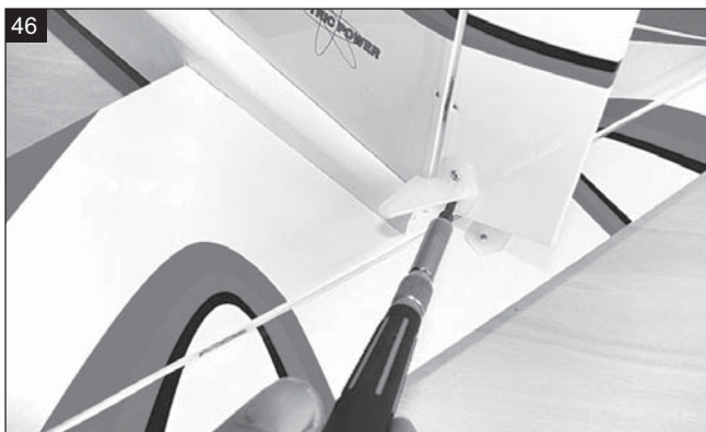
46 Install the rudder control horn.
