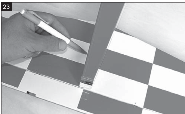
Mark the shape of the fuselage onto the bottom of the horizontal.
