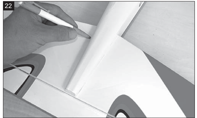
Mark the shape of the fuselage onto the top of the horizontal.
