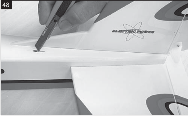
Remove the covering from the slot.
