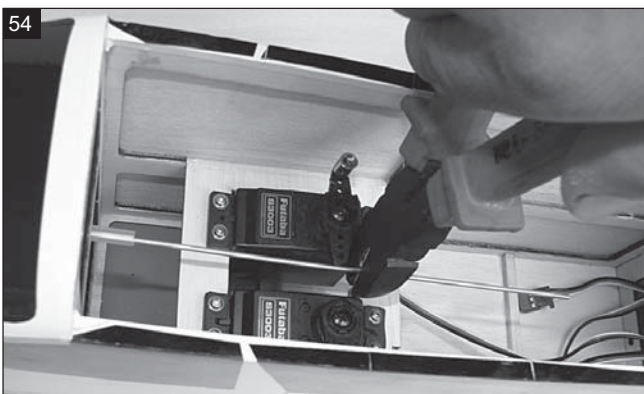
Cut away the rudder pushrod.
