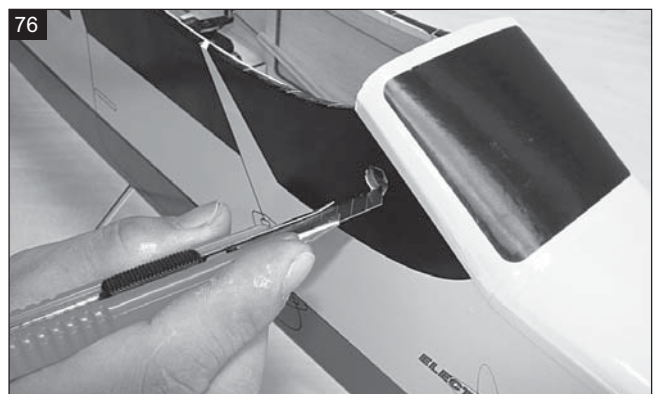
76 Remove the covering from four holes on the both side of the fuselage.
