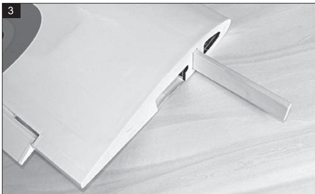
Glue the wing joiner to the wing.
