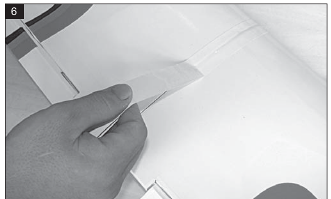
Apply the trim tape to the center section on the top and the bottom of the wing where they join.
