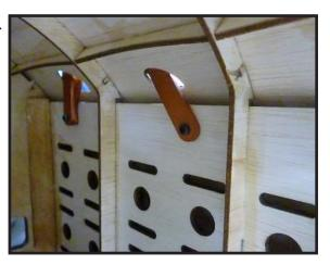
Get the middle number 4 strut and install it on the fuselage.
