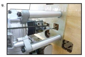
Position the engine with the drive washer (197mm) forward of the firewall.
