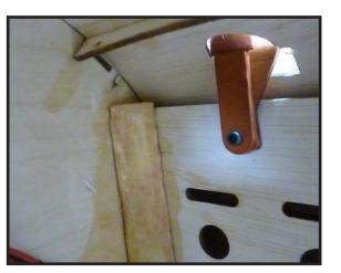
Get the middle number 3 strut and install it on the fuselage.
