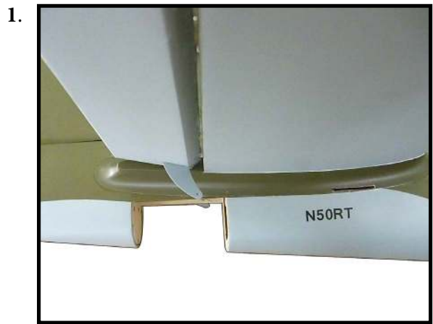
ELEVATOR PUSHROD HORN INSTALLATION
