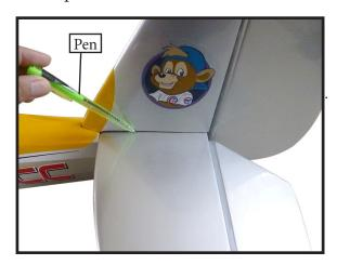
5) Remove the stabilizer. Using the lines you just drew as a guide, carefully remove the covering from between them using a modeling knife.
