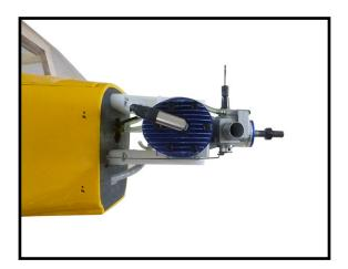
Blow through one of the lines to ensure the fuel lines have not become kinked inside the fuel tank compartment. Air should flow through easily.
