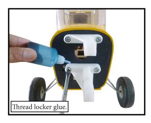
INSTALLING THE STOPPER ASSEMBLY.
