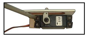
7) Apply 1-2 drops of thin C/A to each of the mounting tabs. Allow the C/A to cure without using accelerator.
