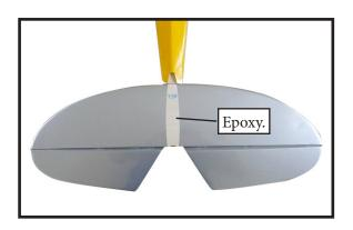
4) Slide the vertical stabilizer back inplace. Using a triangle, check to ensure that the vertical stabilizer is aligned 90° to the horizontal stabilizer.
