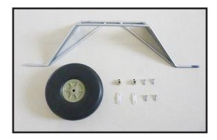
Thread a mounting screw into each of the holes to cut threads in the surrounding wood. Apply a small amount of thin CA to harden the threads make by the screws. Position the landing gear so it rakes forward. Use the screws and landing gear straps to secure the landing gear to the bottom of the fuse-lage.
