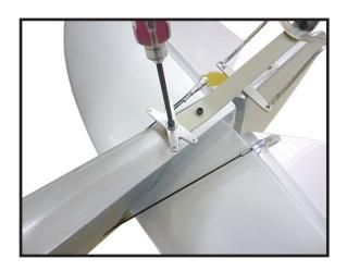
5) Install water rudder control cables.
