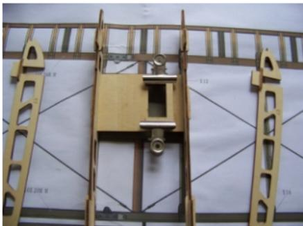
(1) Glue the servo mount "C" type strengthening plate.
