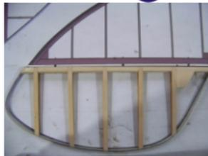
(6) Cover the 1mm plywood sheets on ribs and then joint and glue on the elevator.
