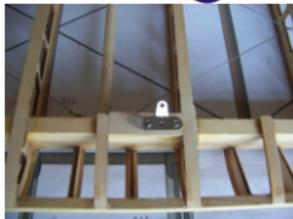
(13) Install the appropriate wood block on the mount of wing strut, and smooth it ,then install the metal parts like the pictures.
