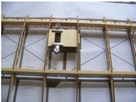
(3) The girders in the kit come with bevel, please notice the installing direction for front and back girders. (Front girder with forward bevel and back girder with backwards bevel.)
