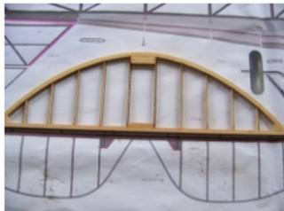
(2) Glue the strengthening plate and ribs. Make sure the top of the ribs (8mm) on the middle of the 5\*10mm batten, reserve 1mm both side for 1mm plywood sheets cover.
