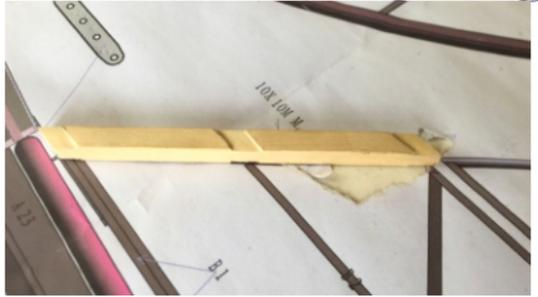
(6) Cut 6 mm deep grooves (both ends and middle, up and down side) on the vertical fin front batten like the picture, in order to glue 1mm plywood sheet in the grooves.
