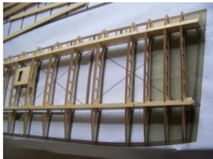
(4) Fix the girders towards to the installation drawing with long steel nails.
