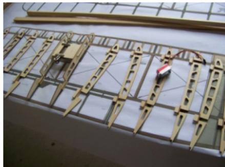
(2) Joint and glue the servo mount on E8 ribs .Insert the strengthening plates and glue them to ribs.
