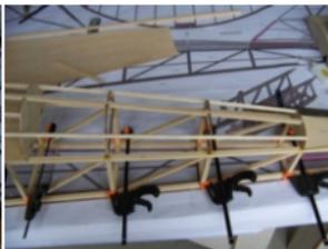
(11) Joint and glue the bulkhead and battens according to the installation drawing.
