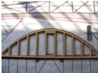
(3) Cut 1mm deep grooves for glue 1mm plywood sheet on ribs.
