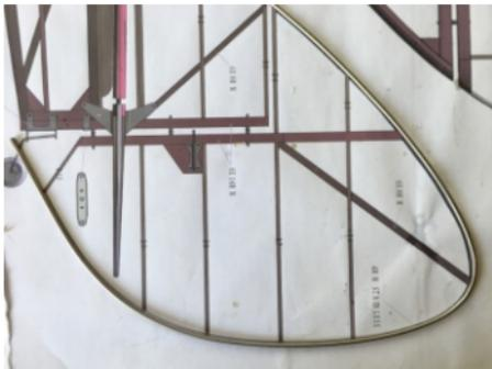
(3) Bending the 4mm stainless steel tube.
