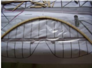
(1) Joint the retral frame of fuselage with battens according to the installation drawing. Then connect it on the fuselage.
