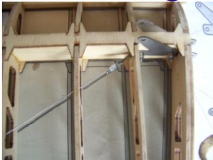
(11) Joint rib E1. And fix the wing on the installation drawing again, then pull  $\phi$  0.8mm steel wires.
